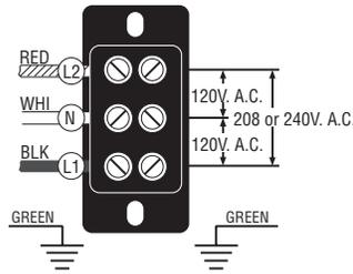
**Model 35** requires 3-wire, grounded service rated 120/208 or 120/240 volts ac, 20 amp, single phase, 60 Hz. Proceed as follows:
