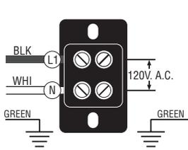
**Model 20** requires 2-wire, grounded service rated 120 volts ac, 20 amp, single phase, 60 Hz. Proceed as follows:
