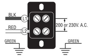
**"A" & "B"** models require 2-wire, grounded service rated 200 volts ac or 240 volts ac, 20 amp, single phase, 50 Hz. Proceed as follows:
