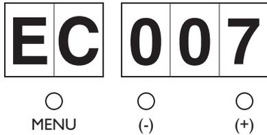
Tank Temp Sensor Failed
