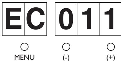
Power Supply Failure
