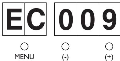
Heat Sink Temp Sensor Failed
