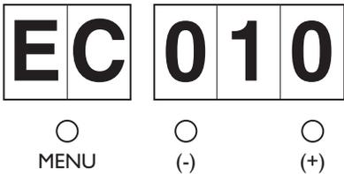
Switch Board Failure
