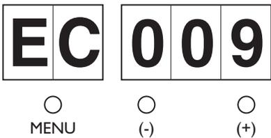
Heat Sink Temp Sensor Failed
