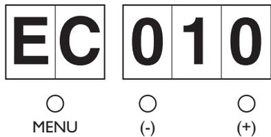
Switch Board Failure
