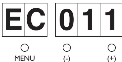
Power Supply Failure
