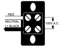
**MODEL RT25B** requires 2-wire, grounded service rated 100 volts ac, 20 amp single phase, 50 Hz.
