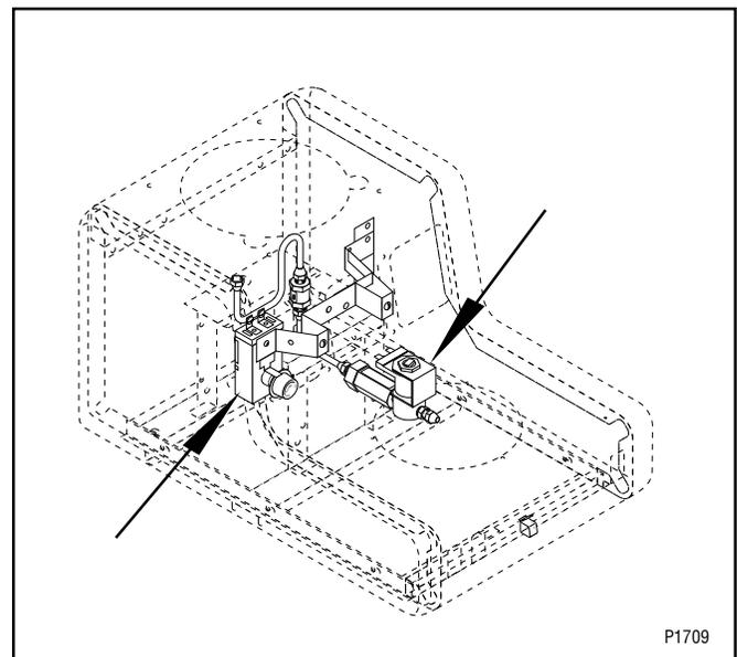
**NOTE** - Bunn-O-Matic recommends 1/4" copper tubing for installations of less than 25 feet and 3/8" for more than 25 feet from the 1/2" water supply line. A tight coil of copper tubing in the water line will facilitate moving the brewer to clean the counter top. Bunn-O-Matic does not recommend the use of a saddle valve to install the brewer. The size and shape of the hole made in the supply line by this type of device may restrict water flow.
