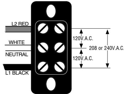
**MODELS OT35 & RT35** require 3-wire, grounded service rated 120/208 or 120/240 volts ac, 20 amp, single phase, 60 Hz.
