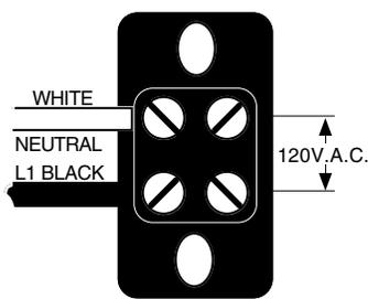
**MODELS OT15 & 20** require 2-wire, grounded service rated 120 volts ac, 15 or 20 amp respectively, single phase, 60 Hz. Model 15 has an attached cordset.
