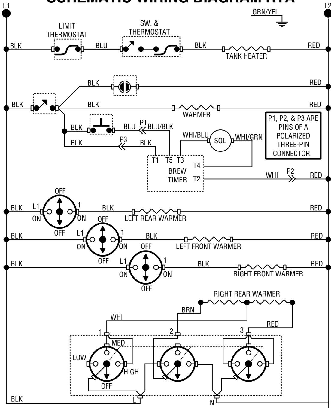
P1, P2, & P3 ARE PINS OF A POLARIZED THREE-PIN CONNECTOR.
