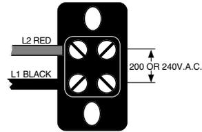
**MODELS OTA, RTA & RT35B** require 2-wire, grounded service rated 240 volts ac or 200 volts ac, 20 amp single phase, 50 Hz.
