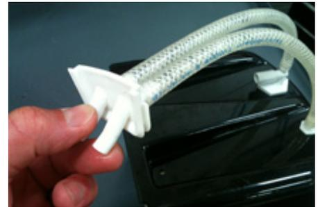
3. Route the tubes from the motor cover together and connect to hopper fitting.
