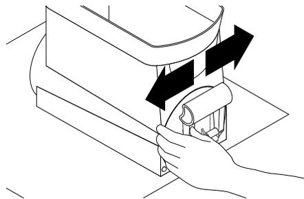
6. **Caution:** The faucet valve is under spring tension. Spread one side of the handle first, then the other and disconnect from the hopper.
