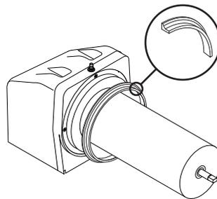
7. Install each hopper seal over the flange at the rear of the cooling drums as shown.
