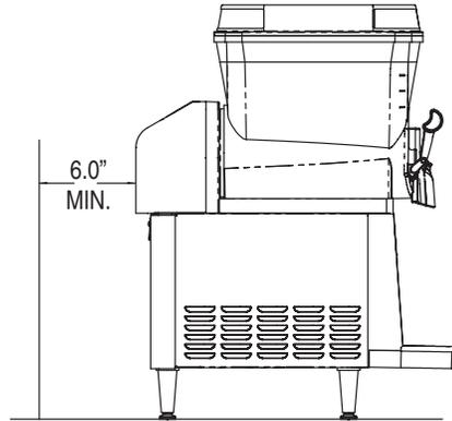
1. Set the dispenser on a sturdy counter top. The dispenser requires a minimum of 6.0" air clearance at the rear of the dispenser. For optimum performance, **do not** let warm air from surrounding machines blow on the ULTRA dispenser.
