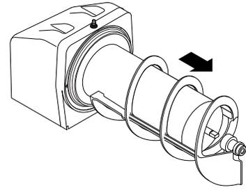
4. Pull the auger from the cooling drum.
