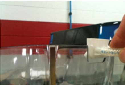
4. Slide hopper fitting into place in the slot on the hopper.
