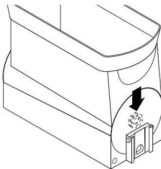
8. Remove the auger nose bushing from inside the hopper.
