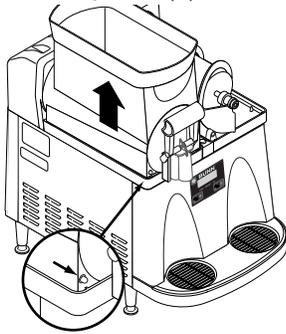
2. Depress the hopper lock plunger. Lift the hopper up slightly.
