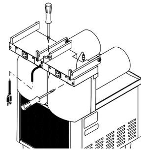
5. Tighten support rod from top of platform. Retighten motor cover screws.
