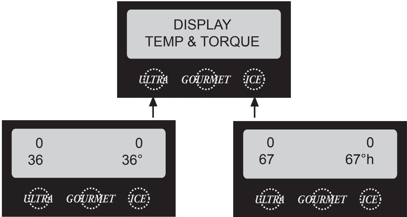
**NOTE:** ULTRA-1 models will display Barrel Temperature and Torque readings on the left side of the display.
