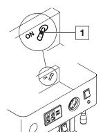
Place the programming lever (1), located under the boiler cover of the machine, in the ON position.
