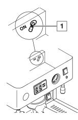
Place the programming lever (1), located under the boiler cover of the machine, in the ON position.
