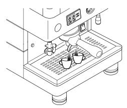
Insert a pod in the filter holder and attach it to the group, tightening firmly.
