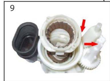
9 Turn the shaft **CLOCKWISE** till it stops to insert the upper gear. Then turn the shaft all the way **COUNTER CLOCKWISE**.
