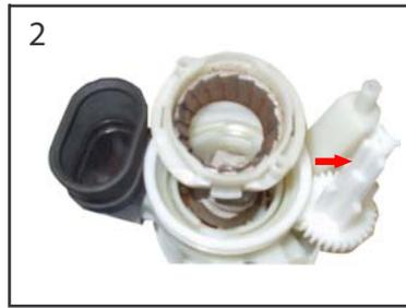
2 Turn the white shaft clockwise till it stops. Remove the upper part of the grinder by pulling it upwards.
