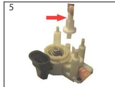
5 Turn the white shaft counter-clockwise till it stops. Pull to remove it.
