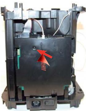
Loosen the screws as illustrated, slide out the electrical connection and remove the card guard.
