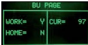
Press the ESPRESSO button to move the unit to Work position. When the unit is in position, the WORK indication changes from "N" to "Y", the absorption current must be less than 200mA without the brewing unit on, and less than 300mA with the brewing unit on.
