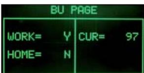
When the unit is in position, the WORK indication changes from "N" to "Y", the absorption current must be less than 200mA without the brewing unit on, and less than 300mA with the brewing unit on.
