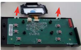
Remove the electrical connections between the card and the display and release the card from the support.
