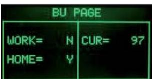
Press the COFFEE button to shift the unit into Home position. When the unit reaches HOME position the indication changes from "N" to "Y", the absorption current must be less than 200mA without the unit or less than 300 mA with the unit on.
