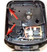
Unscrew the screws shown and slide out the left side body.
