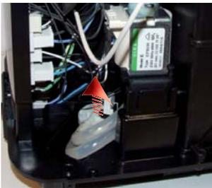
Lift the flow meter out of the casing assembly and remove the electrical and water circuit connections.
