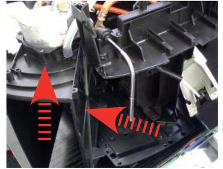
Loosen the screws as illustrated and release the insert in the bottom of the body to obtain easy access for valve disassembly
