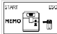
Insert the milk carafe and press the "MEMO" button to start the brewing and save. Press "MEMO" to exit.
