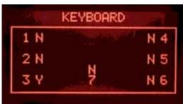
The letter next to it changes from N to Y only when a button is pressed. By pressing buttons 1, 3, 4, 6 the display color changes from GREEN to RED. By pressing buttons 2, 5, the display color changes from GREEN to YELLOW. Button 4 must be pressed at the end only once as when pressed it moves to the next page.
