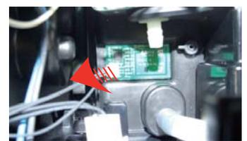
Loosen the screw as illustrated and remove the capacitive sensor glued to the seat.
