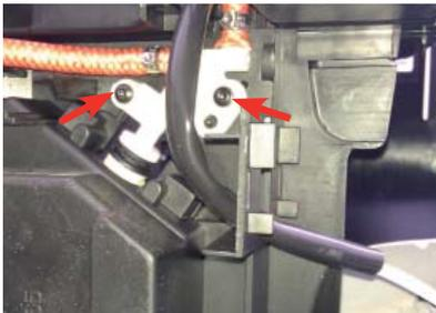
Loosen the screws as illustrated, remove the hydraulic connections and take out the valve
