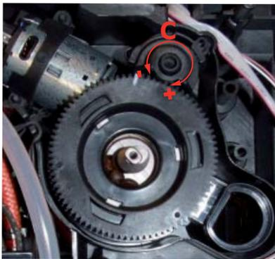
To adjust grinding further, the engineer can work directly on the coffee grinder by pressing and turning the ring nut (C) shown. (clockwise + to increase the particle size of the coffee and anticlockwise - to decrease it).
