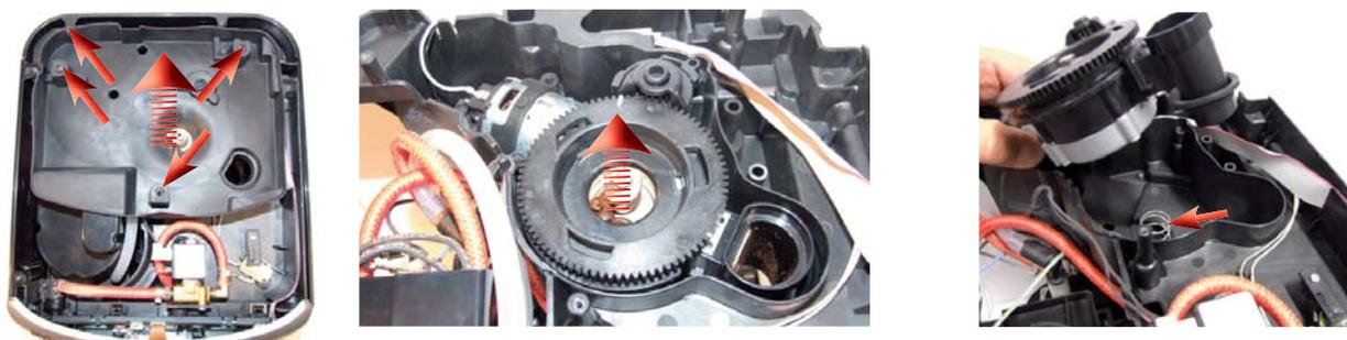
Loosen the screws as illustrated and remove the sound insulating cover. Raise the coffee grinder and remove the connections.
