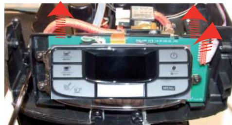
Disconnect the electrical connections and unhook the card support.
