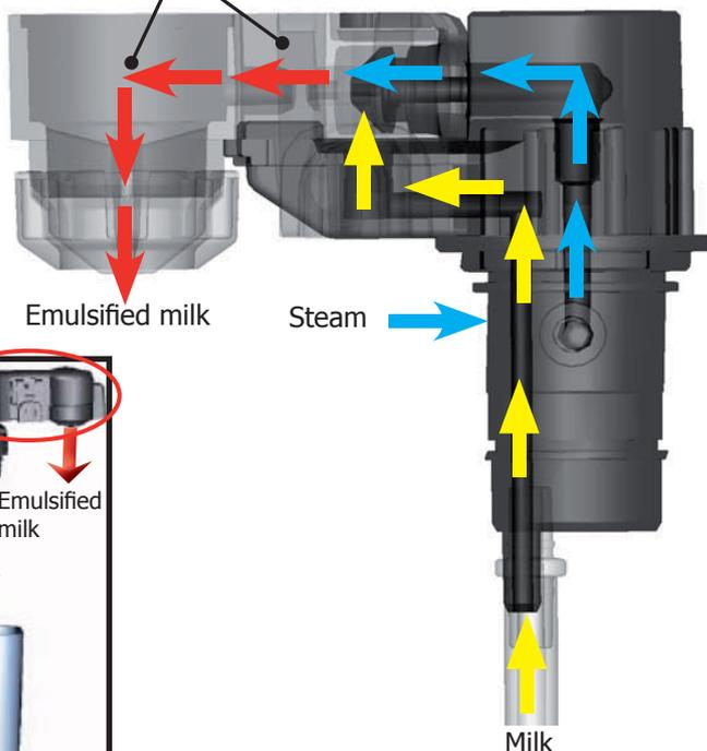
The steam passes through the pipe creating a sucking effect that pulls the milk upwards
