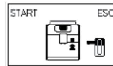
Insert the milk carafe and press the "MEMO" button to start the brewing. Press "MEMO" to exit.
