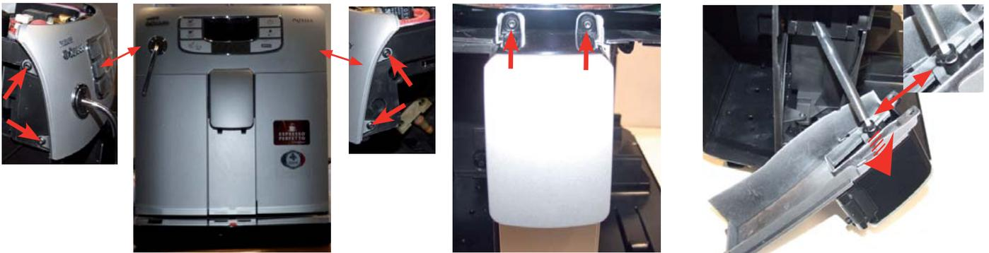
Unscrew the screws as illustrated and remove the front panel to access the screws which fix the dispenser cover into place.
