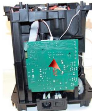
Slide the card off the support and disconnect the electrical connections.
