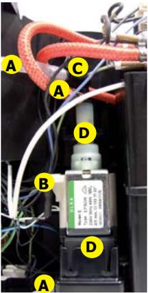
Disconnect the water circuit connections (A) and electrical connections (B), loosen the safety valve (C) and slide the pump off the brackets (D).
