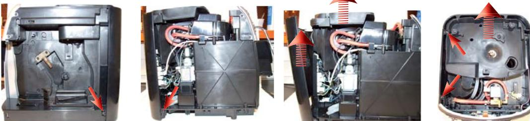
Loosen the screws as illustrated, slide out the rear body and the sound insulating cover of the coffee grinder.
