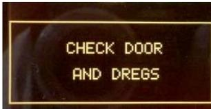
If the following screen appears it means that the dreg drawer is not correctly inserted, or that the side door is not completely closed. The screen will disappear only after the drawer has been inserted or the door closed.
