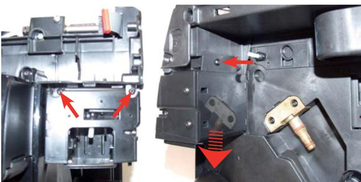
Unscrew the screws (highlighted) and release the milk jug plug body assembly
