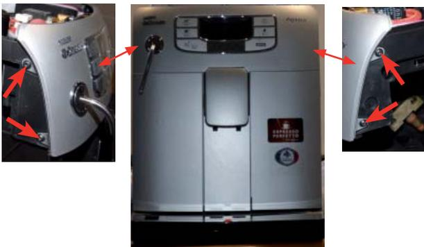
Loosen the screws as illustrated and remove the front panel.
