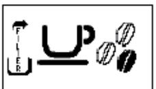
The machine needs the "INTENZA+" filter to be replaced.
