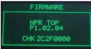
Shows the version of the firmware loaded and the internal checksum (it gives univocal traceability)
