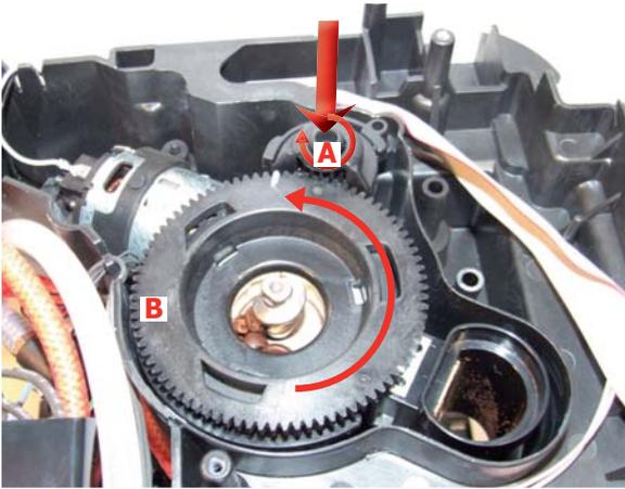
To extract the top support of the appliance, press on the grinding adjustment spindle (A) and turn the support anticlockwise until it unhooks.
