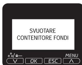
Remove the dregs drawer. Note: The dregs drawer must only be emptied when requested by the machine and with the machine on.
