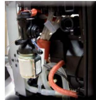
Disconnect the electrical and water circuit connections
