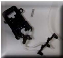
Remove the Teflon pipe support assembly
