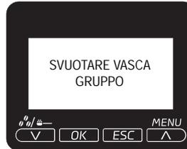
Open the front hatch and empty the drip tray underneath the brewing unit. You should also empty the dreg drawer, as the dregs counter will also be reset when the machine is switched on.
