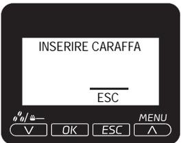
An operation has been selected that requires dispensing from the milk container. Insert the milk container. Press "ESC" to cancel the procedure
