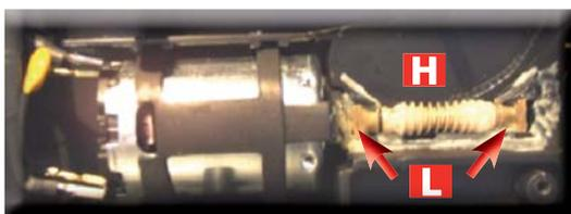
When replacing the motor and the transmission shaft, make sure the guide runners (L) are in the right position. Grease the shaft thoroughly and evenly.
