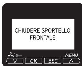
For the machine to become operative, the service hatch must be closed
