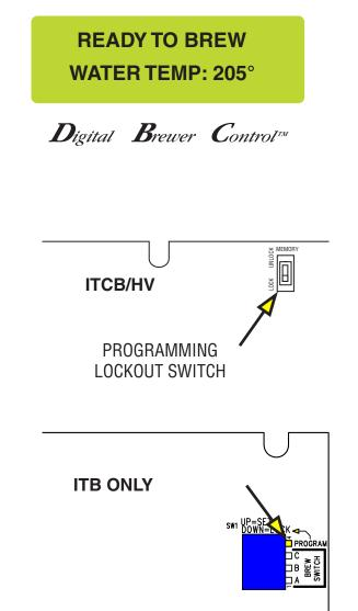
This screen will be shown when the brewer is ready for use. The screen displays the water temperature in the tank. When the water in the tank reaches the correct set temperature, the display will change from **HEATING** to **READY TO BREW.**
