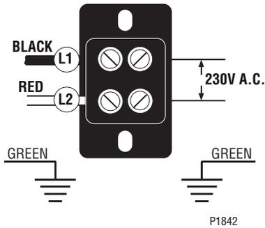
**SRUA-CE Models** require 2-wire, grounded service rated 230 volts ac, 30 amp, single phase, 50 Hz.
