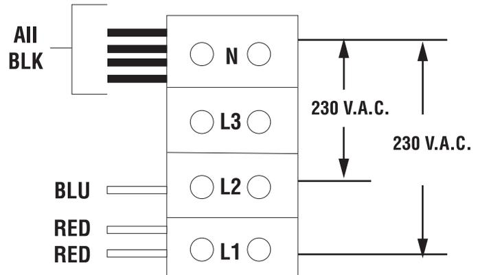
**U3A** Requires 4-wire, 3-phase grounded service rated 400 volts ac, 15 amp, 3 phase, 50 Hz.
