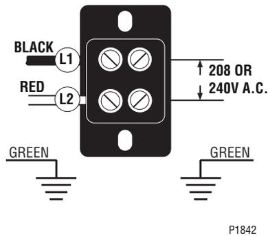
**SRU Models** require 2-wire, grounded service rated 208 or 240 volts ac, 30 amp, single phase, 60 Hz.
