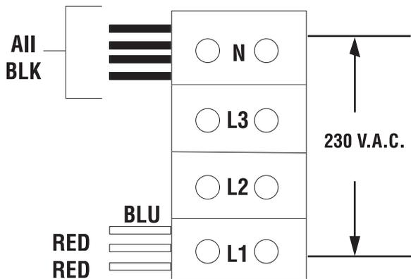
**U3A** Requires 2-wire, grounded service rated 230 volts ac, 32 Amps, single phase, 50 Hz.
