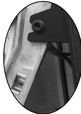
Loosen the 4 Front Panel Screws
