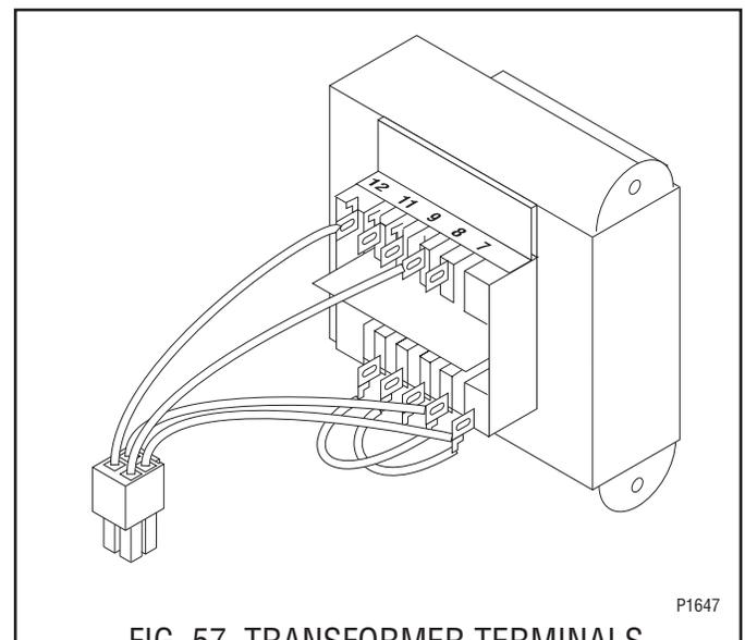
FIG. 57 TRANSFORMER TERMINALS
