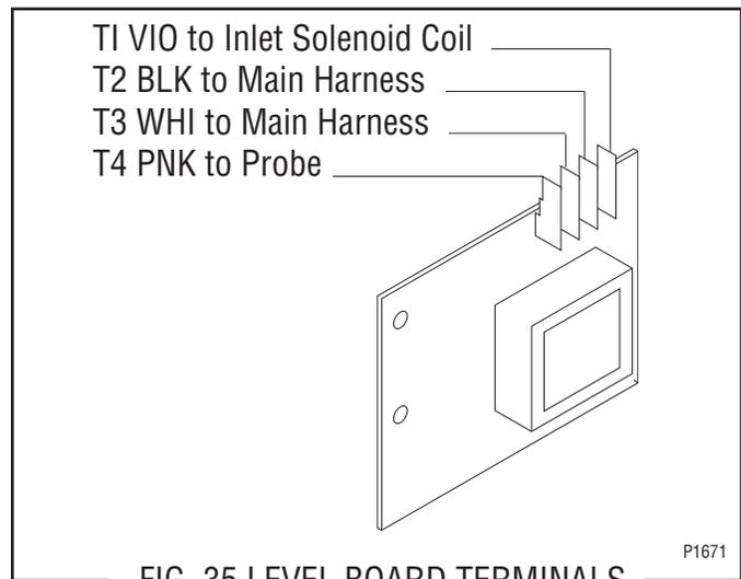
FIG. 35 LEVEL BOARD TERMINALS
