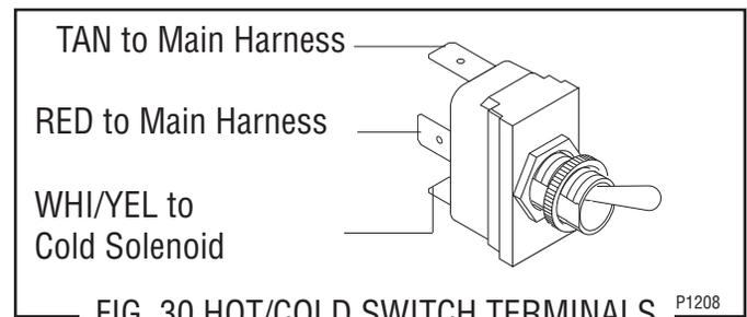
FIG. 30 HOT/COLD SWITCH TERMINALS
