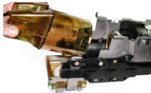
FIG. 4 BREWING CYLINDER BEING REMOVED
