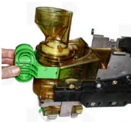
FIG. 3 FEEDER AND COFFEE VALVE BEING REMOVED
