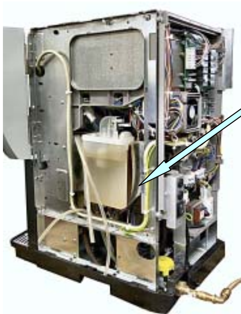
SIDE VIEW - AIR-BREAK SIDE (WITHOUT PROTECTIVE CASING)
