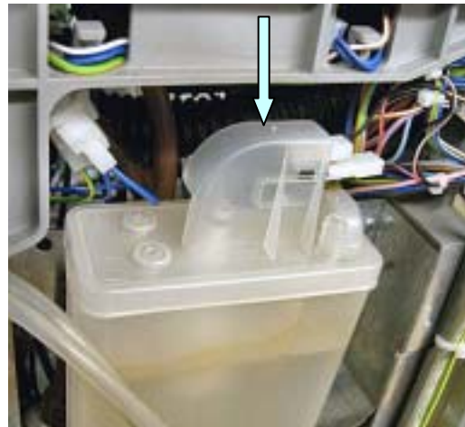
DETAIL OF WATER LEVEL MICRO-SWITCH
