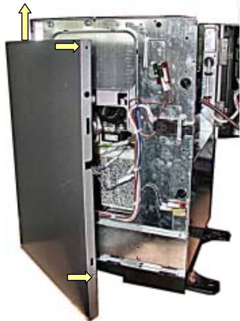
Slightly lift the casing to slide out the upper fasteners
