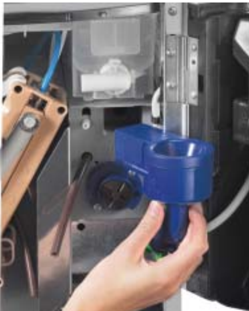
MIXERS WITH EXTERNAL PARTS SUBJECT TO DAILY HYGIENE BEING REMOVED
