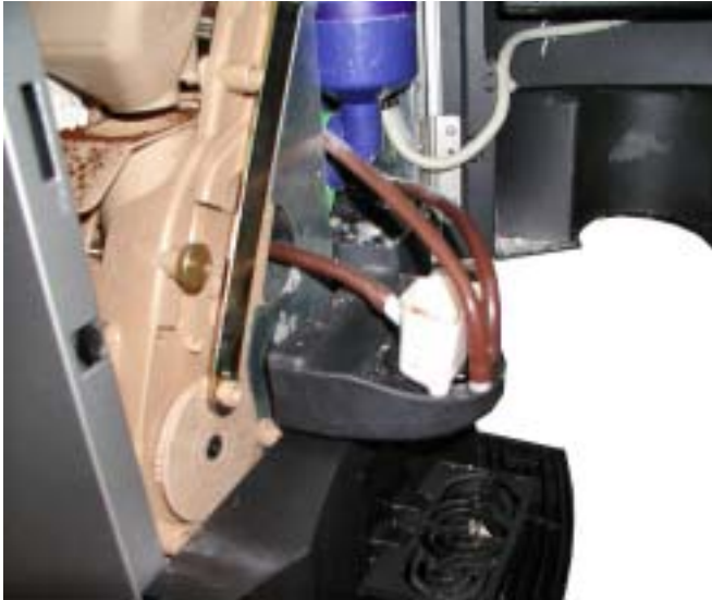
SPOUTS ASSEMBLY EXTERNAL VIEW WITH DETAIL OF COFFEE SPOUT WITH SPLIT OUTLET TO OPTIMISE QUALITY AND TO PERMIT DISPENSING OF DOUBLE COFFEE
