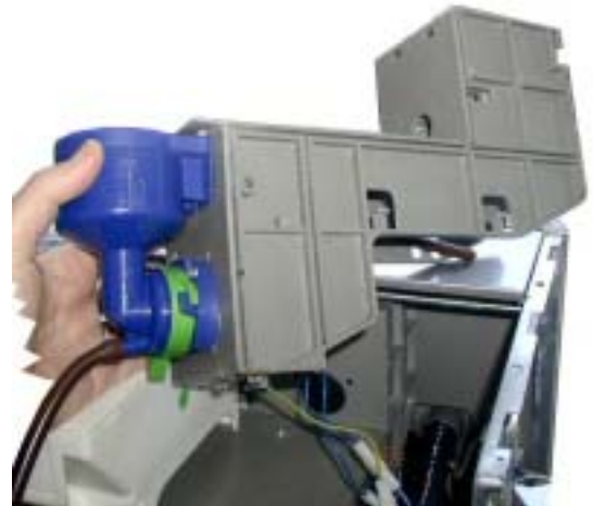
MIXER RATIOMOTOR ASSEMBLY BEING REMOVED FROM ITS SEAT
