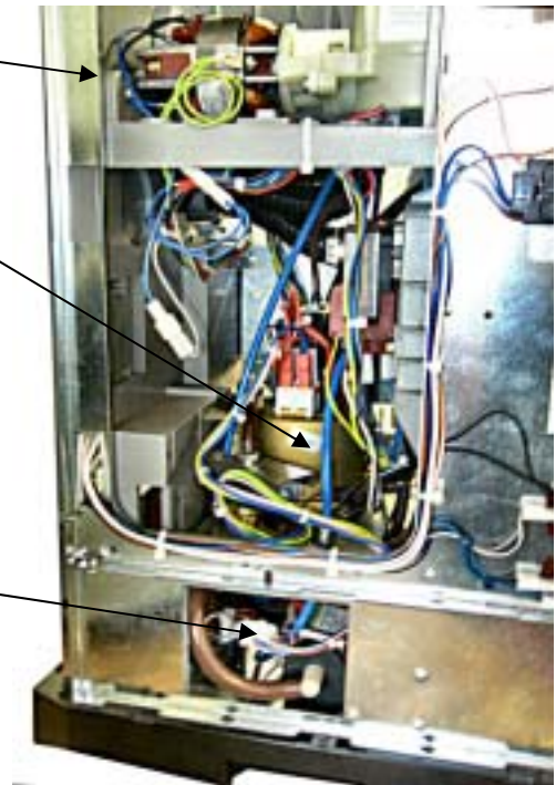
SIDE VIEW WITHOUT PROTECTIVE CASING - ESPRESSO BOILER SIDE
