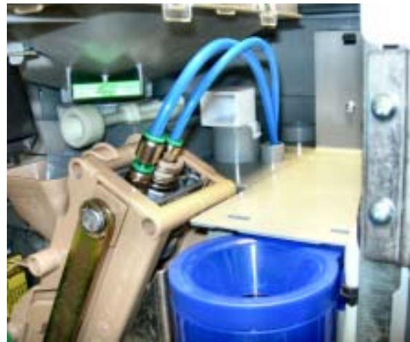
DETAIL OF TUBE CONNECTIONS, ADJUSTMENT OF BREWING CHAMBER AND WATER INLET FOR COFFEE BREWING
