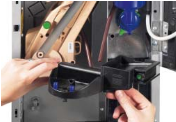
DETAIL OF SUPPORT TRAY BEING REMOVED
