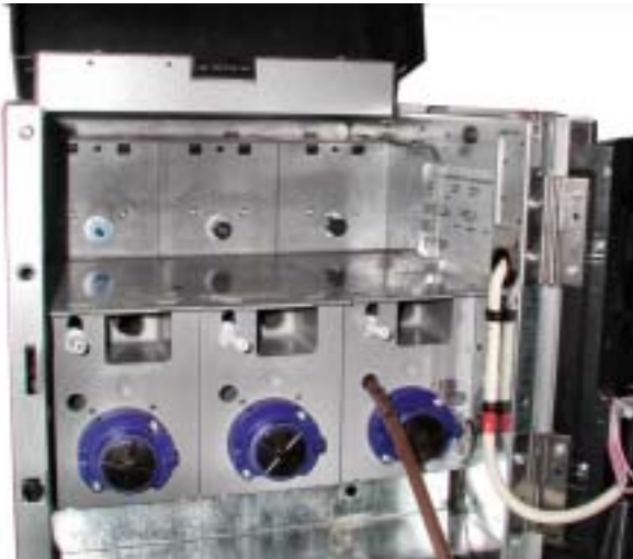
MIXERS WITH EXTERNAL PARTS SUBJECT TO DAILY HYGIENE BEING REMOVED
