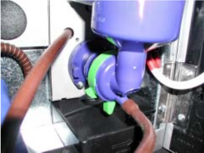
TRAY UNDER THE MIXER BEING REMOVED
