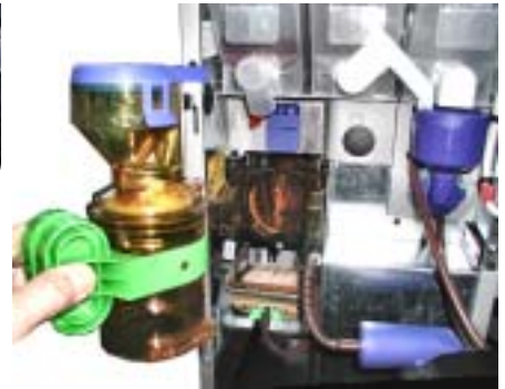
PRESSING THE GREEN PINCER WITH YOUR FINGERS, REMOVE THE BREWING CHAMBER APPLYING A FIRM ACTION
