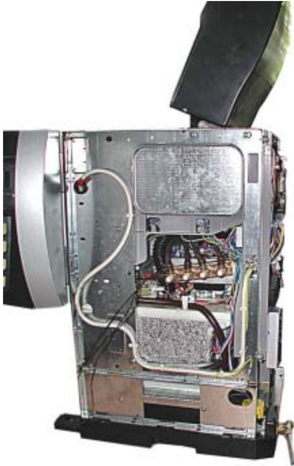
SIDE VIEW WITHOUT PROTECTIVE CASING - INSTANT BOILER SIDE (Only for INSTANT VERSION or FRESH BREWER)
