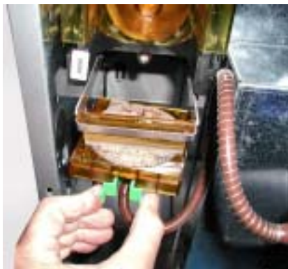
PRESSING WITH YOUR FINGERS THE TWO TABS LOCATED AT THE BASE OF THE FILTER HOLDER, REMOVE THE FILTER HOLDER ASSEMBLY APPLYING A FIRM ACTION
